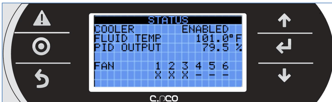
System Status Page – PLC Fan Staging Option
